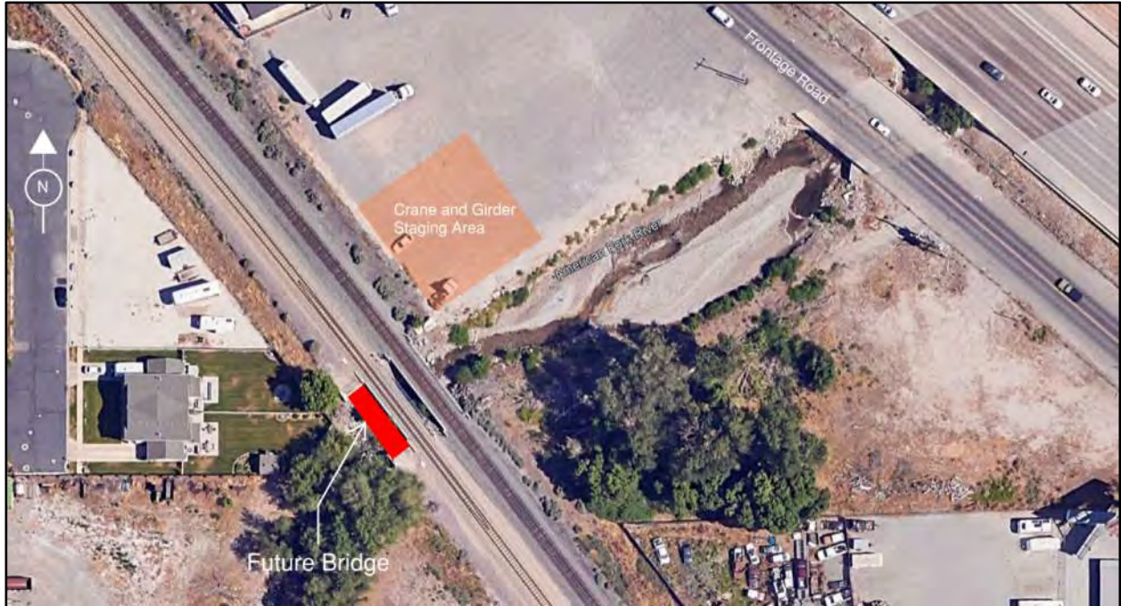
Figure 4 - Potential Crane and Girder Staging Area
