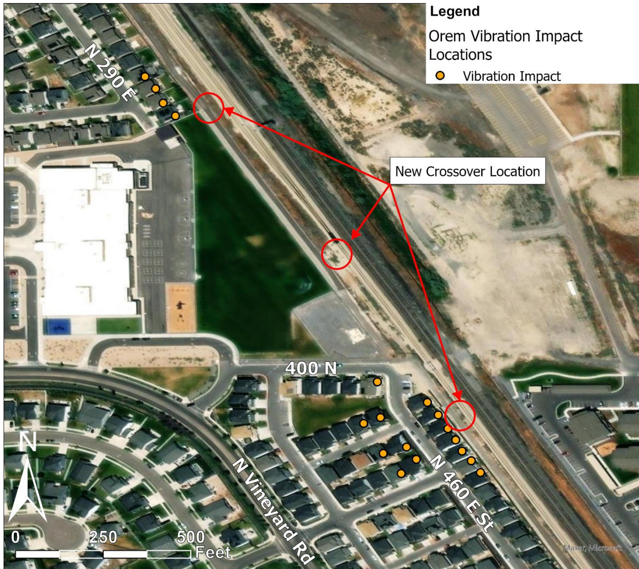
Figure 5. North of Orem Double Track Project
